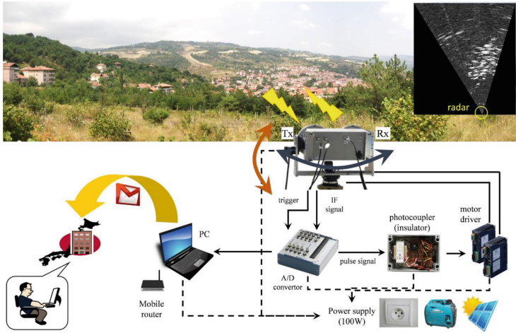
Fig. 1. Conceptual diagram of the ground-based radar system developed.
